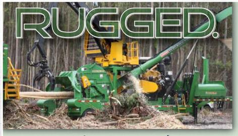
Precision Whole Tree Chippers are built stronger than the competition, and have a reputation for trouble-free service. They have rugged frame construction, oversized stabilizers, air compressors, trash separators, and more powerful fans that pack more chips per van.
