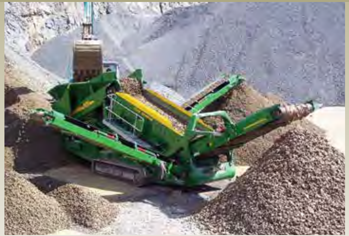
A McCloskey International R155 crushing mixed aggregates.
